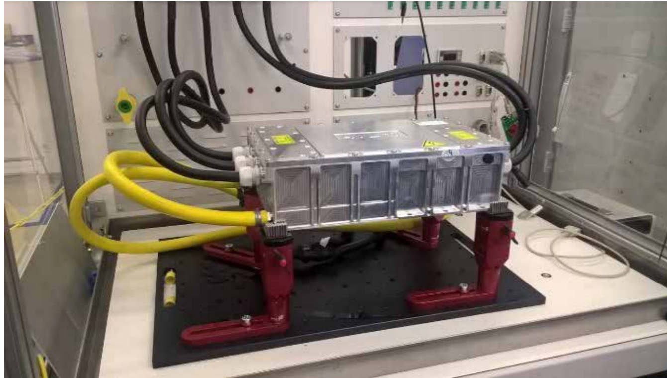
Fig. 34 shows the HF inverter Power HiL test setup
