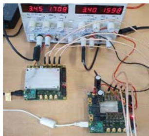
Fig. 37 shows the FHJ Hardware-in-the-Loop demonstrator. Two interconnected ZYNQ Ultrascale+ systems: One emulating at high frequency the e-machine and the inverter and the second one executing the control algorithm
