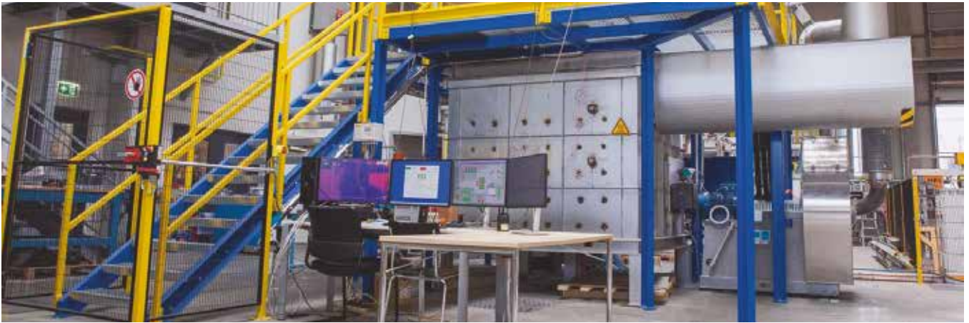
ICPIH – Inductive Coupled Plasma for Industrial Heating
